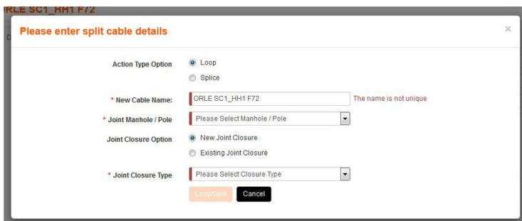
If you **Splice** the cable then a full new Joint Closure will be created in the Manhole you selected, with patch cords automatically joining each new section with Splice Joints.
